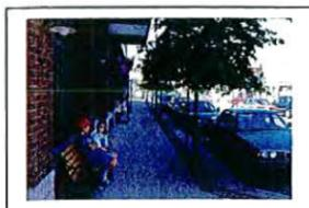
**On-Street/Parallel Parking:** provides a separator between vehicular and pedestrian traffic; utilizes cartway as an “aisle”; (with “overflow” parking to the rear or side of buildings); promotes effective “traffic calming” by slowing down the speed of vehicles, especially along narrower streets
